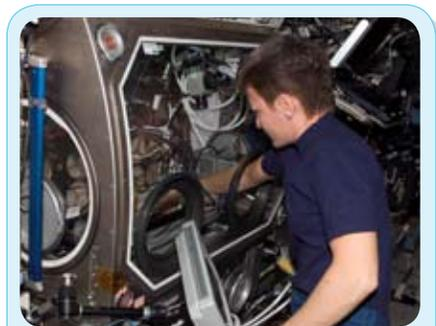
Astronaut Peggy Whitson works at the Microgravity Science Glovebox in the Destiny laboratory of the ISS.
