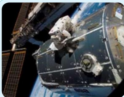
Mission specialist Hans Schlegel works on the outside of the Columbus laboratory module, built by the European Space Agency. Columbus has ten racks for experiments that can be controlled from the station or the Columbus Control Centre in Germany.
